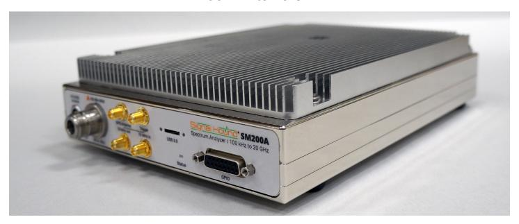
The SM200A is a high-performance spectrum analyzer and monitoring receiver. Tuning from 100 kHz to 20GHz, the analyzer has 160MHz of instantaneous bandwidth, 110dB of dynamic range, 1THz/sec sweep speed at 30kHz RBW (using Nuttall windowing), and phase noise performance that is low enough to contribute less than 0.1% error to EVM measurements and rival even the most expensive spectrum analyzers on the market.
