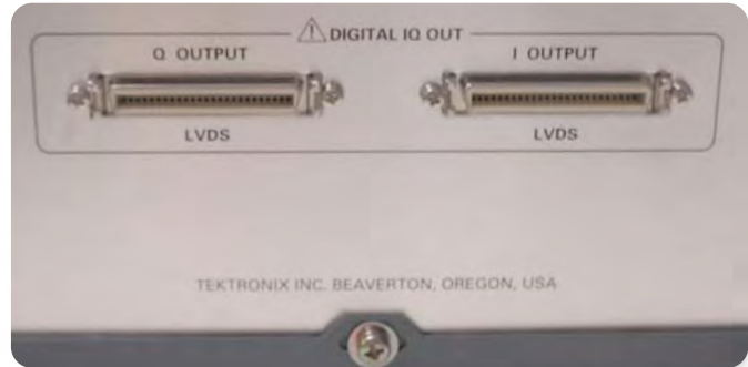
Figure 25. Equipped with LVDS ports, extracting I-Q records continuously in real-time is easily accomplished with the RTSA.
