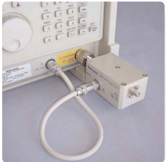
Figure 11. Optional RTSA preamplifier lowers the analyzer noise floor and adds 20 dB of gain, improving reception performance. The preamplifier is powered directly from the RTSA.
